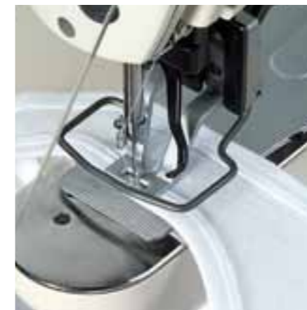
M type (Bartacking shoulder of running shirt)
