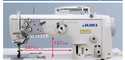
The machine is suited to sew car seats, sofas and bags, provided with dramatically improved workability and functions required for sewing large products and extra heavy-weight materials.
